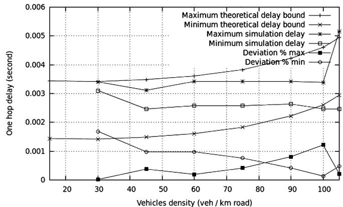
**Fig. 3.** One hop delay simulation results function of vehicles density and compared to theoretically deduced bounds.
