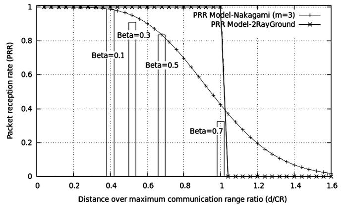
**Fig. 2.** Packet reception rate corresponding to the optimal relay selection function of distance over communication range ratio.
