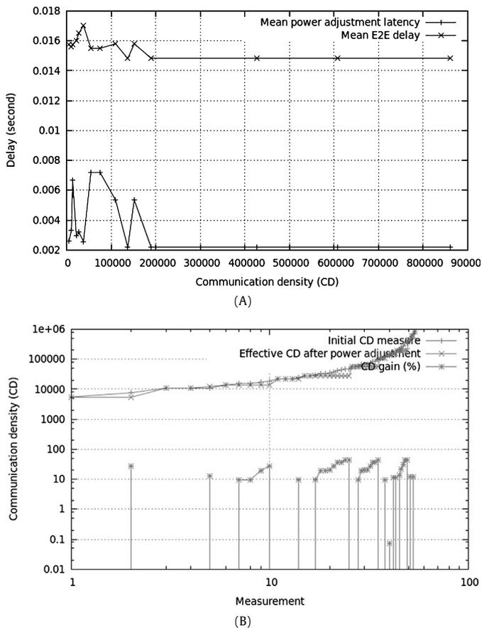
Fig. 7. (A) MORS power adjustment latency and E2E delay. (B) Power adjustment effect on the CD.
