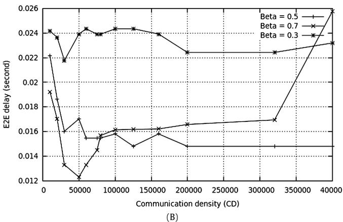
**Fig. 4.** (A) End-to-end MORS mean delay compared to other solutions while varying CD. (B) End-to-end MORS mean delay varying  $\beta$  proportionality parameter and subjected to different CD.
