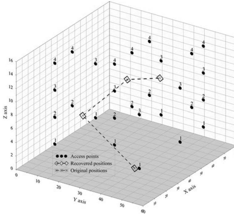
Figure 2. Recovered target positions using 3D-CS method in ideal conditions.
