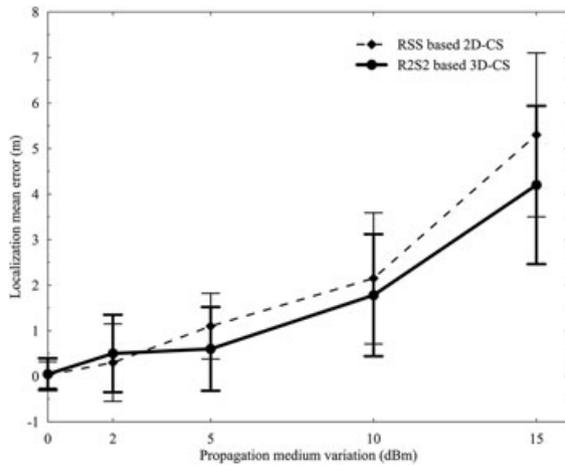
Figure 3. Influence of the propagation medium variation on the localization mean error for 2D-CS and 3D-CS methods.
