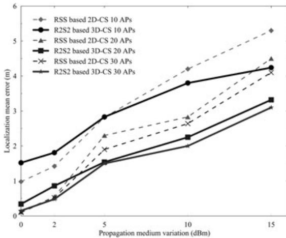
Figure 6. The localization mean error determined by varying the propagation medium variation and the number of APs using 2D-CS and 3D-CS methods in NLOS condition.
