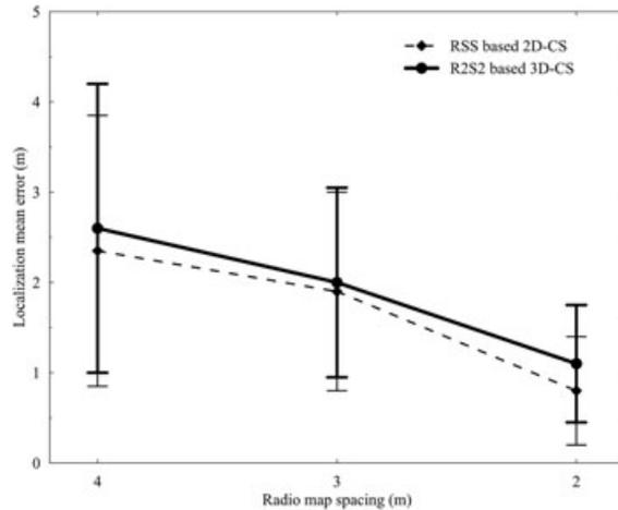
Figure 7. Influence of the radio map spacing on localization mean error.
