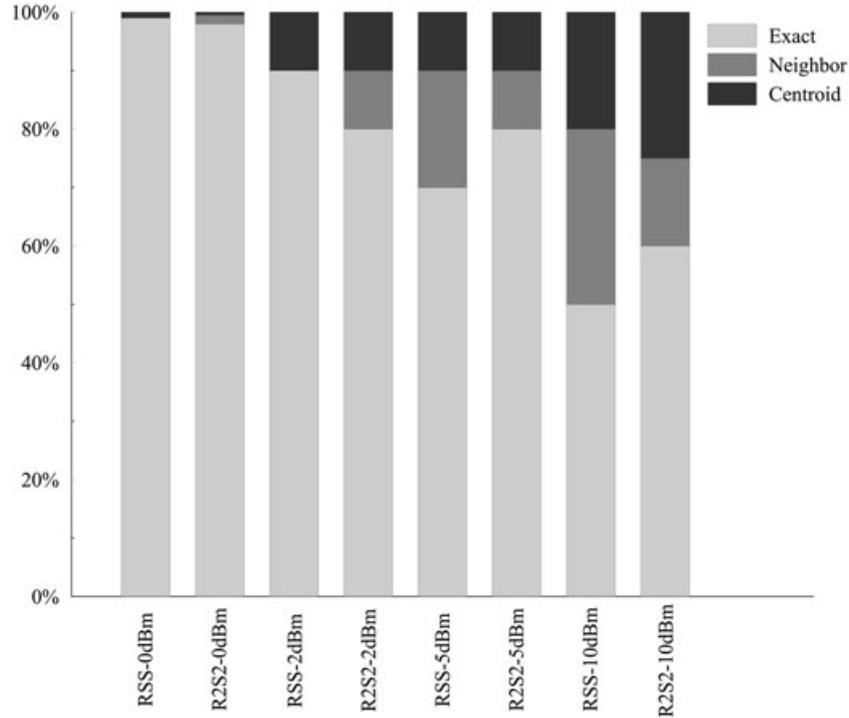
**Figure 4.** Details of recovered positions using RSS and R2S2 metrics with different propagation medium variation levels in LOS condition.
