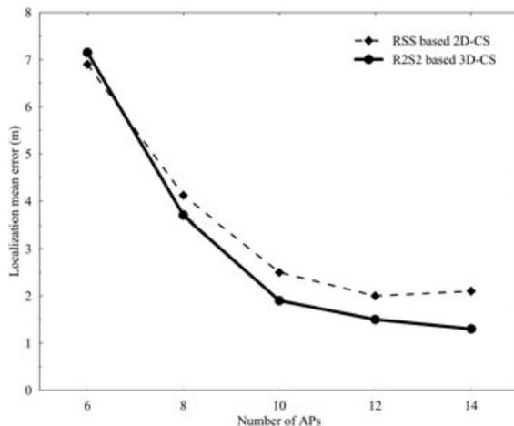
**Figure 9.** Influence of the number of APs on localization mean error determined by experimental results.
