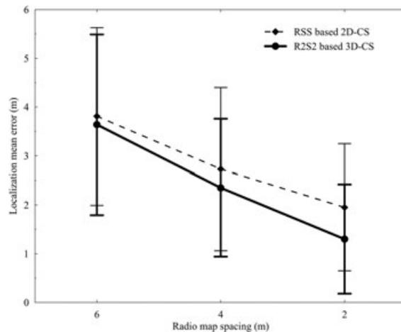
**Figure 10.** Influence of the radio map spacing on localization mean error determined by experimental results.
