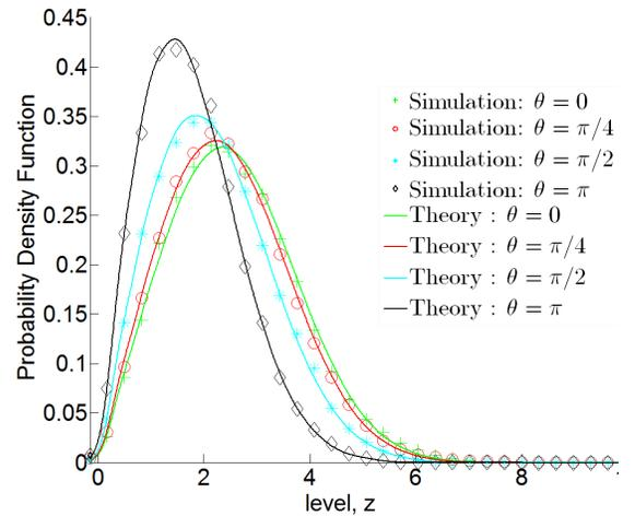
Fig. 2. Variation with respect to  $\theta$  of the first stage process PDF in presence of the LOS components for both channel (1) and channel (2).
