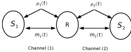
Fig. 1. Asymmetric time-varying two-way relay channel. When it exists,  $m_i(t)$  is the LOS component, and  $\mu_i(t)$  is the scattered or non LOS (NLOS) component that describes the fading in channel ( $i$ ).
