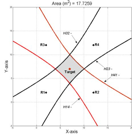
Fig. 6. Intersection area with a RSS Based Localization method.
