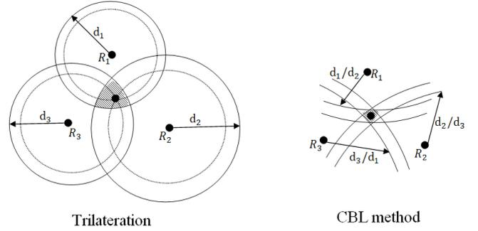
Fig. 2. Illustration of Trilateration and CBL methods.
