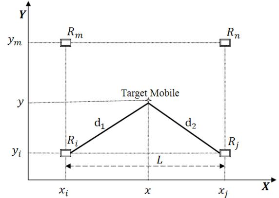
Fig. 3. Illustration of triangulation and CBL methods.
