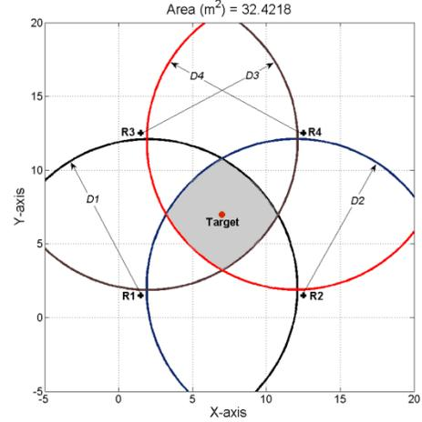
Fig. 5. Intersection area with the Trilateration based localization method.
