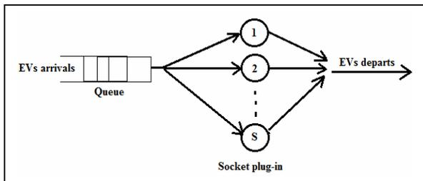
Figure 1: Schematic view of our EV charging model for one EVPSS.
