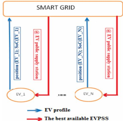
Figure 4: Schematic view of information flow between the Smart Grid and EVs by considering the BA-EVPSS algorithm.
