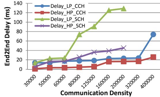
FIG.7. DELAY FUNCTION OF CD IN CCH AND SCH WITH LOW PRIORITY (LP) AND HIGH PRIORITY (HP) IN P2V CASE
