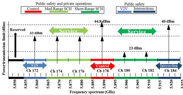
FIG. 1. DSRC FREQUENCY SPECTRUM AND CHANNEL ALLOCATION
