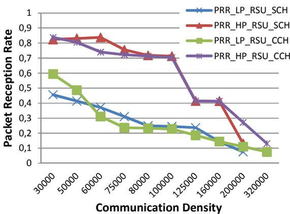
FIG.10. PRR FUNCTION OF CD IN CCH AND SCH WITH LP AND HP IN P2I+I2V CASE
