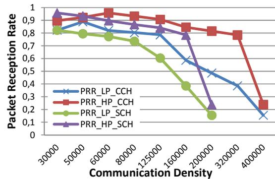
FIG.8. PRR FUNCTION OF CD IN CCH AND SCH WITH LP AND HP IN P2V CASE
