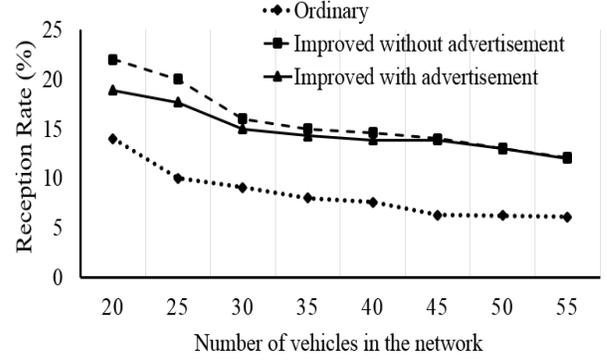
**Figure 6: Reception rates of the proposed scheme vs. standard.**
