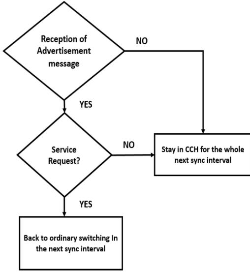
Figure 3: Flowchart of the proposed multi-channel switching.
