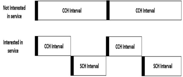
Figure 4: Proposed multi-channel switching.
