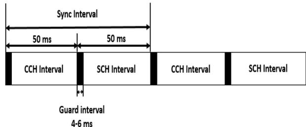
Figure 2: Ordinary multi-channel switching.
