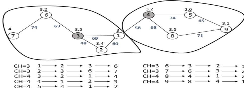
Figure 1 Cluster formation using DCEV (D=3).
