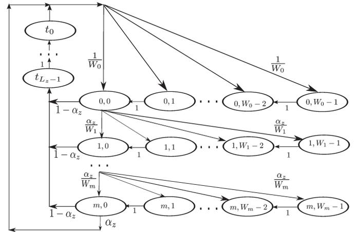
Fig. 2. Markov chain model of the transmitting node for the unslotted IEEE 802.15.4 CSMA/CA.
