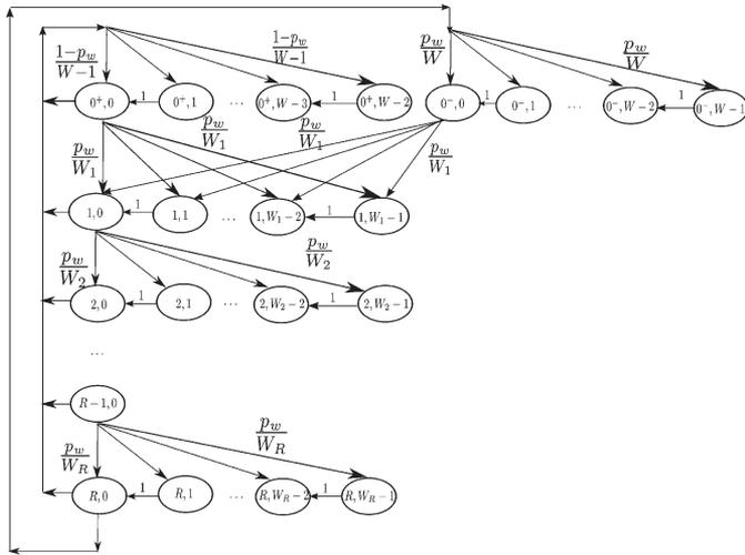
Fig. 1. Markov chain model of 802.11 transmitting node [11].
