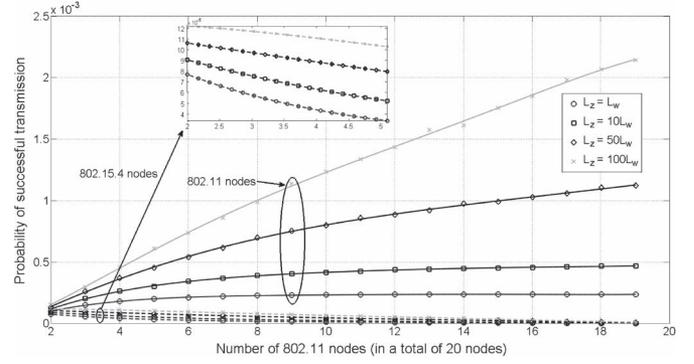
Fig. 3. Probability of successful transmission in the cases  $L_z = L_w$ ,  $L_z = 10L_w$ ,  $L_z = 50L_w$ , and  $L_z = 100L_w$ .
