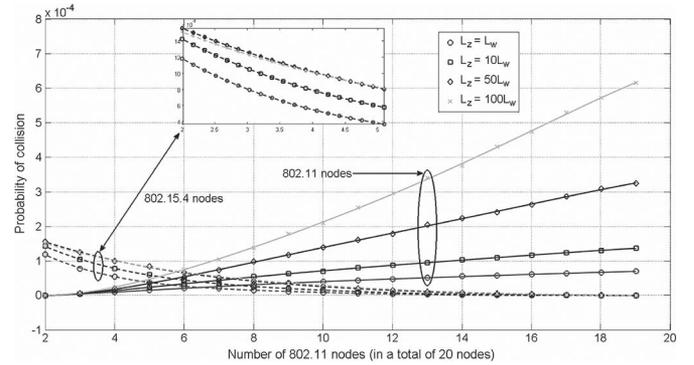
Fig. 4. Probability of collision in the cases  $L_z = L_w$ ,  $L_z = 10L_w$ ,  $L_z = 50L_w$ , and  $L_z = 100L_w$ .
